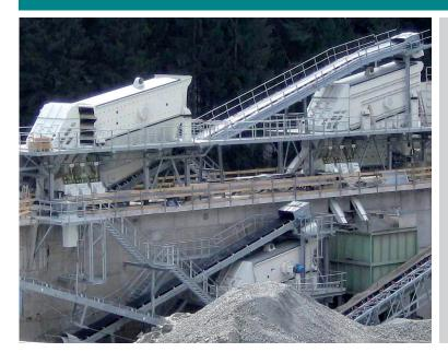
Minimization of investment and operating costs by combining circular vibratory and BIVITEC screening machine
